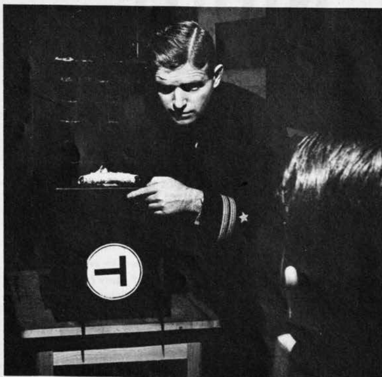
Tests are necessary to determine ability to see in the dark. Student watches a T-shaped plane model on luminous dial and must read correctly the direction it is flying. About 5% have poor night vision.
